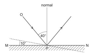
The mirror is rotated through 10°, as shown by the dashed line. The direction of the incident ray OP does not change.
