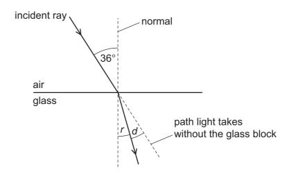
The angle of refraction is r. The angle between the refracted ray and the path the light takes without the glass block is d.
