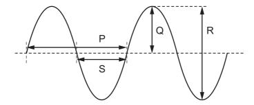
Which lengths represent the amplitude and the wavelength of the wave?
